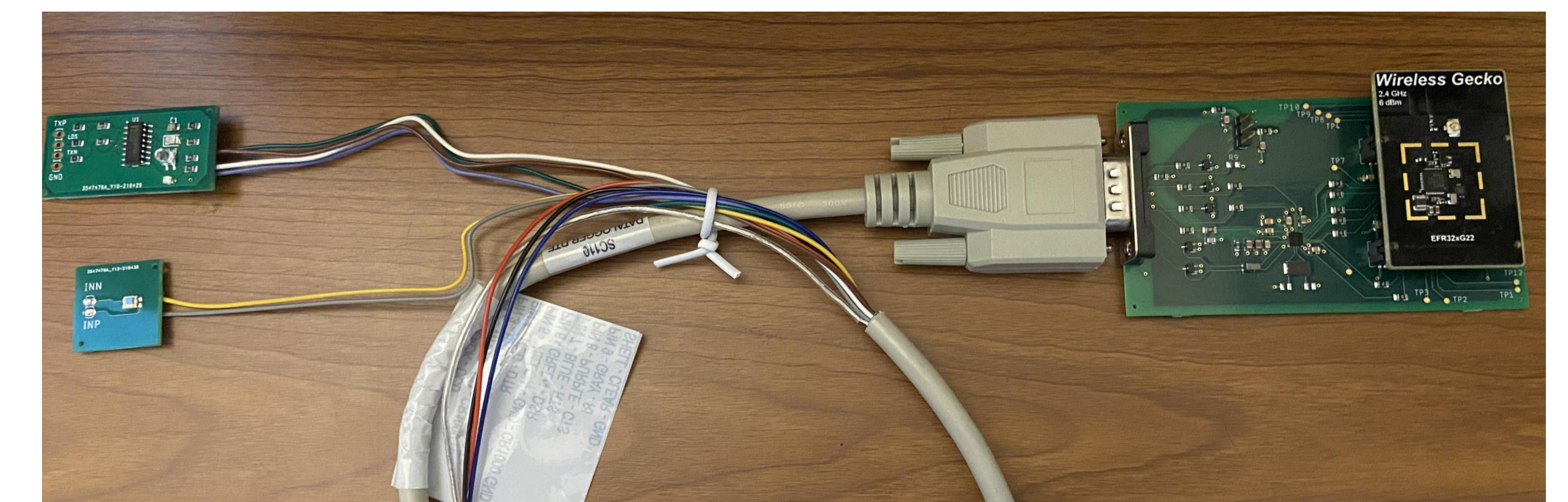
Top left board: LED Controller PCB (Finger Sensor 1) Bottom left board: Photodiode PCB (Finger Sensor 2) Middle cable: DB-9 Connector Right board (green): Main PCB to support AFE4403 and BRD4182A Right board (black): BRD4182A
